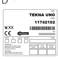
For an easiest repair, replacement or increasement of the existing monitors, fill the indentifying label information.
